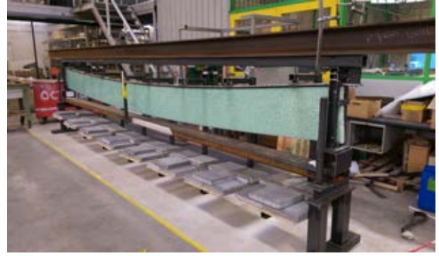
Figure 3: Failure of tempered glass after a bending test
